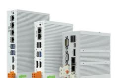
Where demands on computing power and memory are high, WAGO offers the perfect solution with the Edge Computer. It features a 1.91 GHz quad-core Atom processor and is equipped with standard Debian Linux. Users can draw on abundant resources and model entire automation processes on them.
