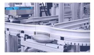
Core components of the montrac<sup>®</sup> system, montrac<sup>®</sup> shuttles are intelligent single or twin-axle conveyors equipped with an on-board power supply. Moving self-centred on the monorail, the shuttles are equipped with state-of-the-art sensors that prevent potential collisions with obstacles or other shuttles.
