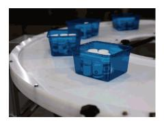
the processing line. The simplified configuration also eliminates the need for straight infeed and outfeed conveyors, which are required in modular belted curves.
