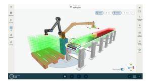
See how the robot moves, check reach, speed, and cycle time before you set anything up on the shop floor. An easy way to plan and launch your automation with confidence.
